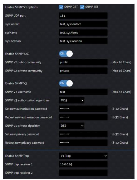
2. Open the snmpb software and navigate to Options/Manage Agent Profiles... and create a new user. Set the Agent Address to the IP address of the PWR4IEC and the port to the SNMP UDP port set in the Web-GUI.
