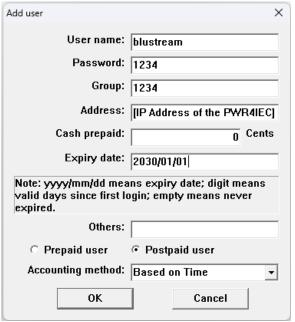
Use the IP address of the PWR4IEC in the address field. Click confirm to add the account
