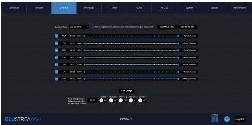
To adjust the logic for any given day, move the blue dots along the timeline to create a highlighted selection: this is when the device will power on. In order to add additional logic (i.e multiple on and off periods), press the + More Schedule button. You can now add additional logic by repeating the steps above.
